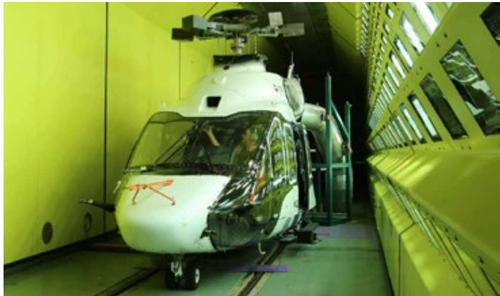
Figure 2 The IWT in Vienna allows icing tests to be carried out at speeds of up to 300 km/h across an icing cross section of 8.75 m 2 ; Image: Rail Tec Arsenal
