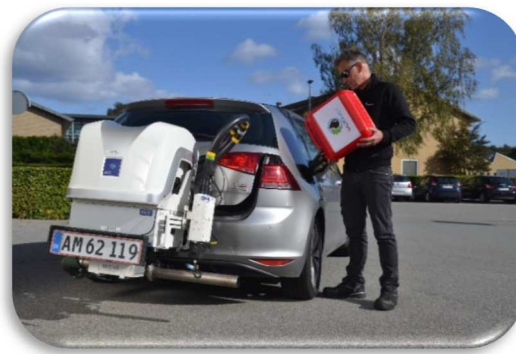
Real driving emission testing with PEMS @DTI
