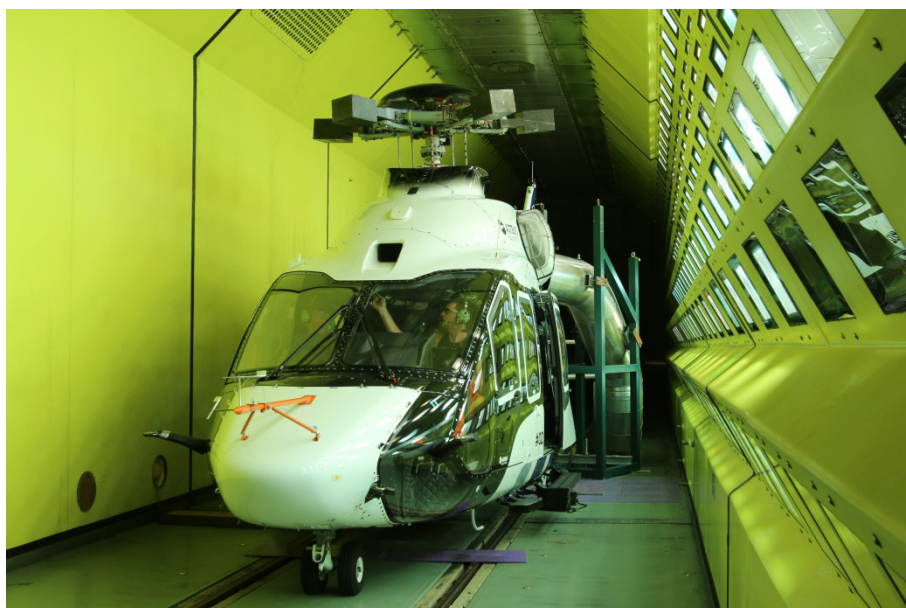
Figure 2: The IWT in Vienna allows icing tests to be carried out at speeds of up to 300 km/h across an icing cross section of 8.75 m 2 ; source: Rail Tec Arsenal
