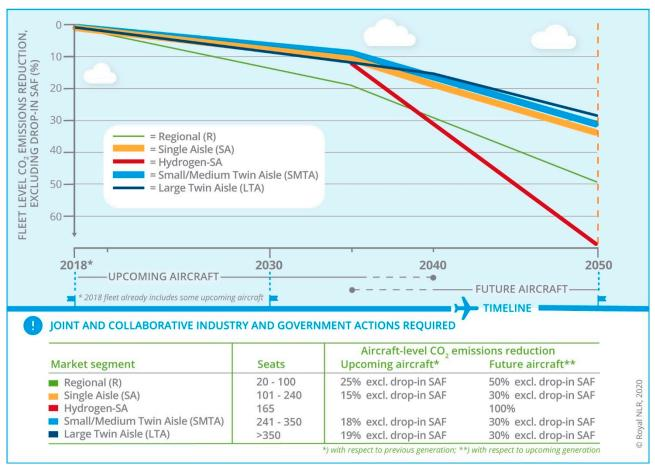
Continued replacement of current aircraft with upcoming models would reduce emissions until 2040. Next-generation future aircraft would yield aircraft-level  $CO_2$  emissions reduction of 30 to 50% compared to upcoming aircraft types. Specifically for the intra-European market, a hydrogen-powered aircraft would enable zero- $CO_2$  flight. At fleet level the  $CO_2$  emissions reduction by upcoming and future aircraft reaches levels of 28 to 67% in 2050.
